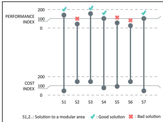
Figure 2. Description of cost/performance for a key module is mapped. Each vertical line represents a module area. The lower dot is the cost and the upper dot is a certain performance of a property.
